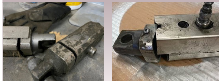
Field Photo of improper installation and operation results
